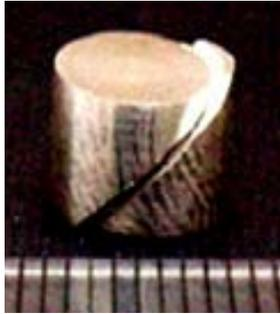
Fig. 2: Sample of the compression test (after the test).
